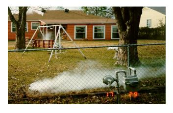
Smoke testing is a very simple process that involves pumping nontoxic smoke into sewer main lines, allowing smoke to seep up through the soil and indicate any cracks or line deterioration which is a source for groundwater to infiltrate our sewer lines and overload the collection and treatment system. The smoke testing program also allows the city to locate
